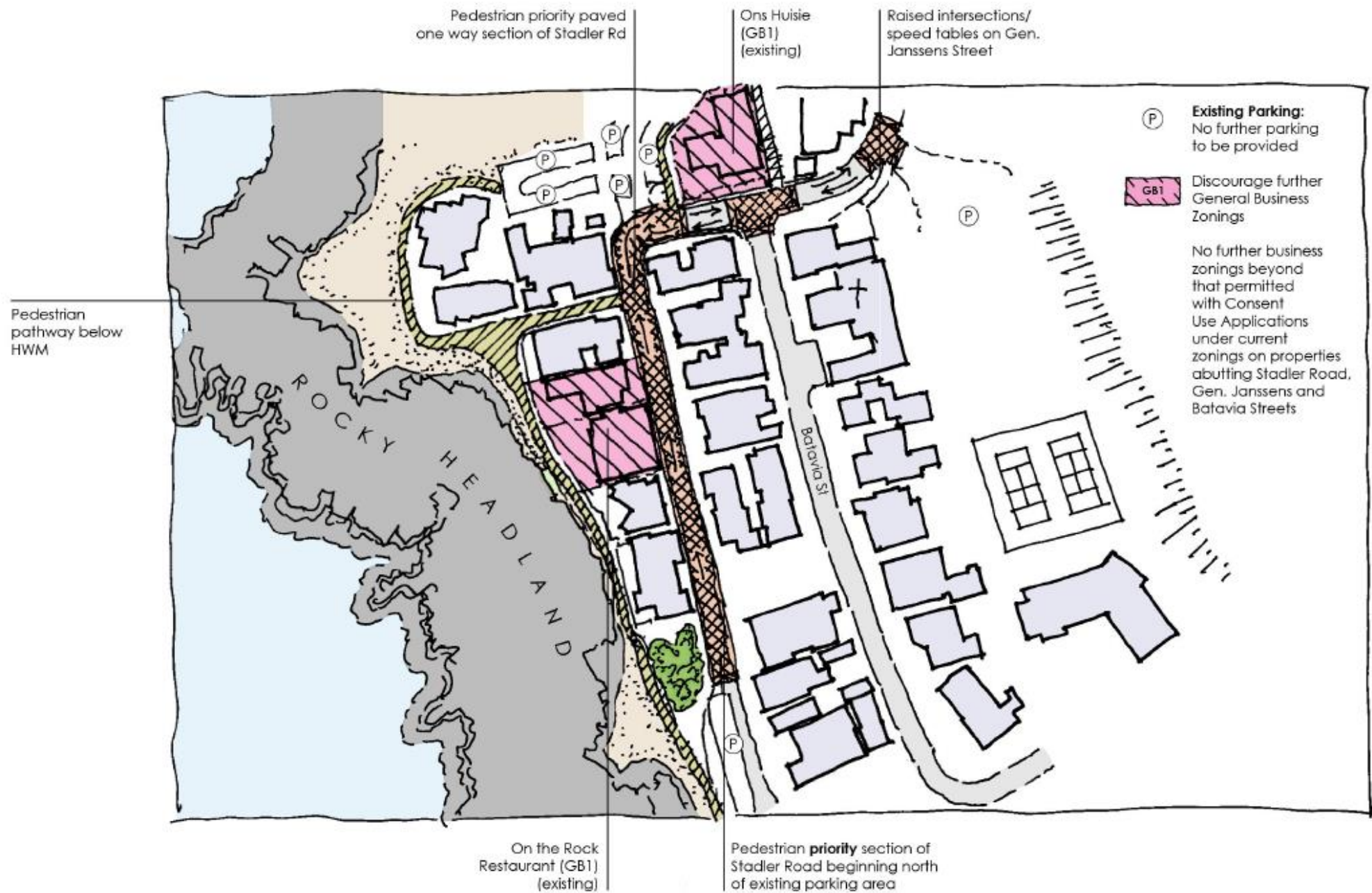
Fig. 7.3.4.30 Proposed extent of Stadler Road upgrading
